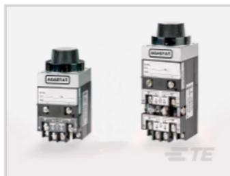
Type of Control: **Knob**Time Delay Relay Input Voltage: **12 VDC**Timing Range (Off-Time): **360 – 3600 seconds**Time Delay Relay Contact Current Rating: **10A@240VAC A**Mode of Operation: **Off-Delay****Features****Product Type Features**
